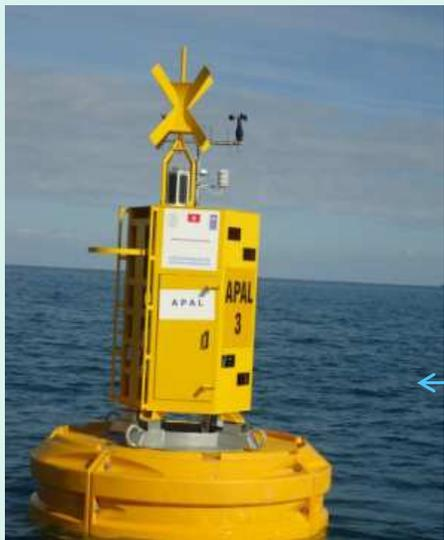
Modem GSM +Antenne
